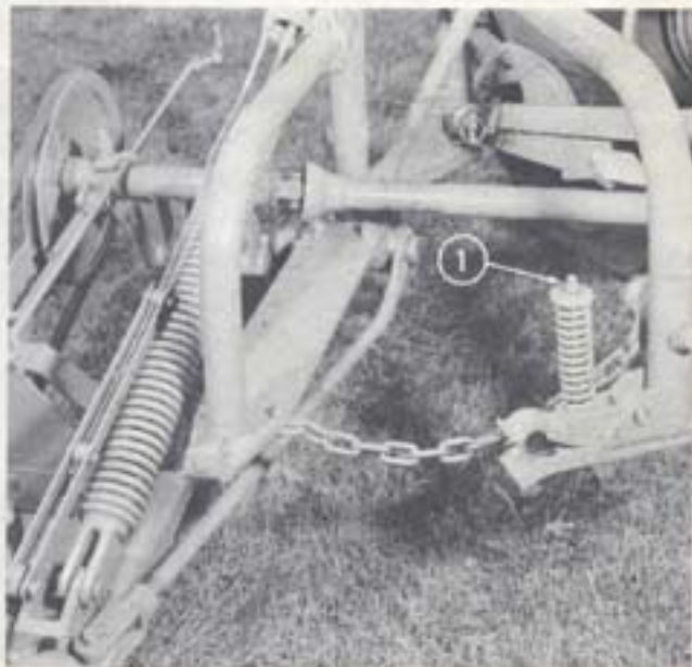
Fig. 24 Safety Release Feature 1. Adjusting nut
