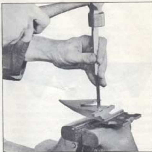
Fig. 50 Replacing Ledger Plates
