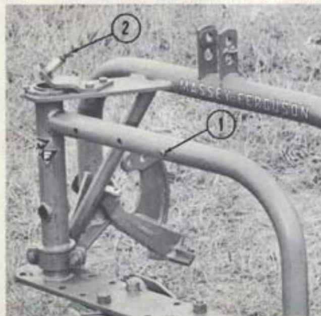
Fig. 57 Roll Pin Inserted 1. Roll pin 2. Lift assembly stud
