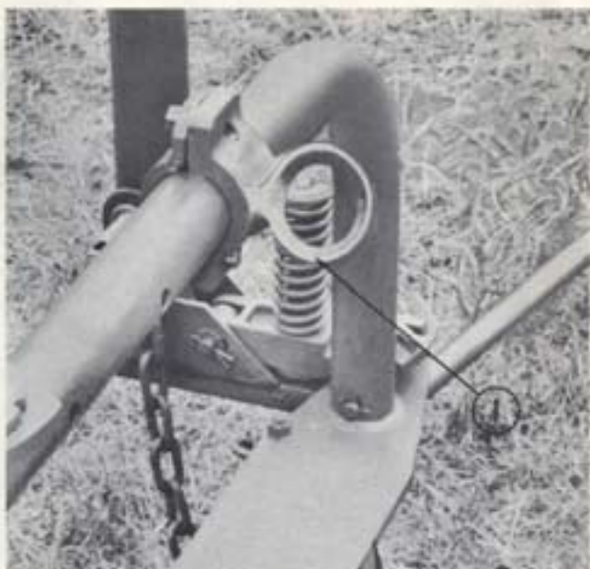
Fig. 58 Bracket for Counterbalance Spring 1. Rear portion of bracket
