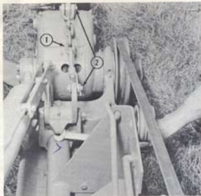
Fig. 25 Checking Gag Linkage
