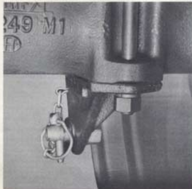
Fig. 7 Stabilizer Bracket Installed
