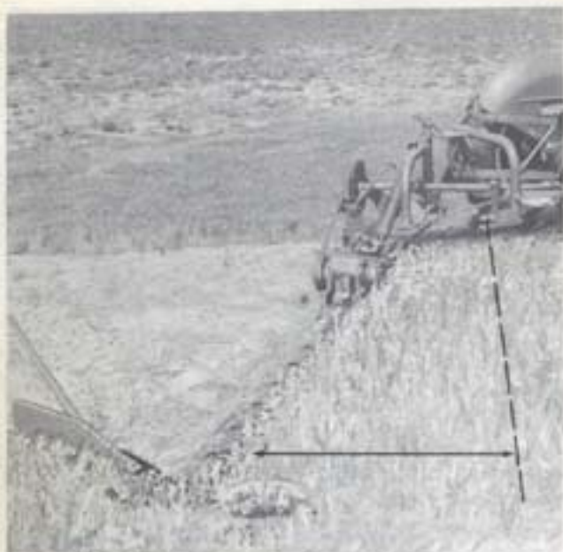
Fig. 19 Cutter Bar "Breaking Back"
