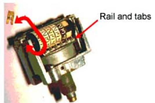
14. Remove two machine screws holding round housing. Invert the assembly and remove the drive disc housing. The reason for inverting is so that you don't allow the drive disc to fall out and stretch or break the clock spring.
