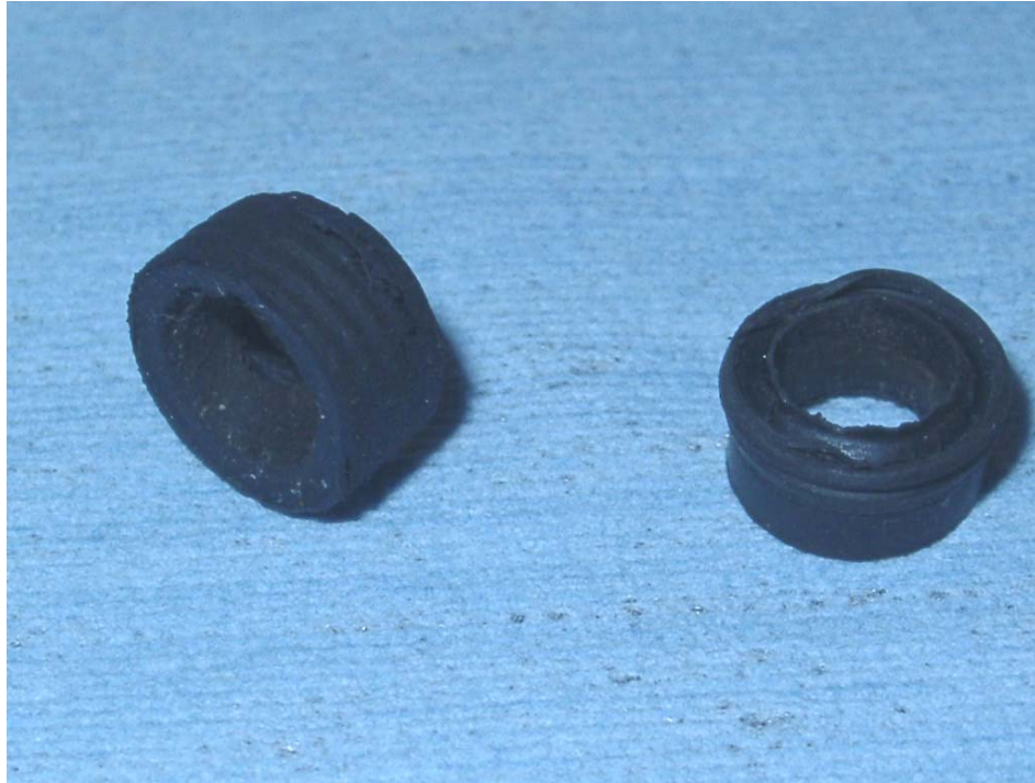
Worn out seals
