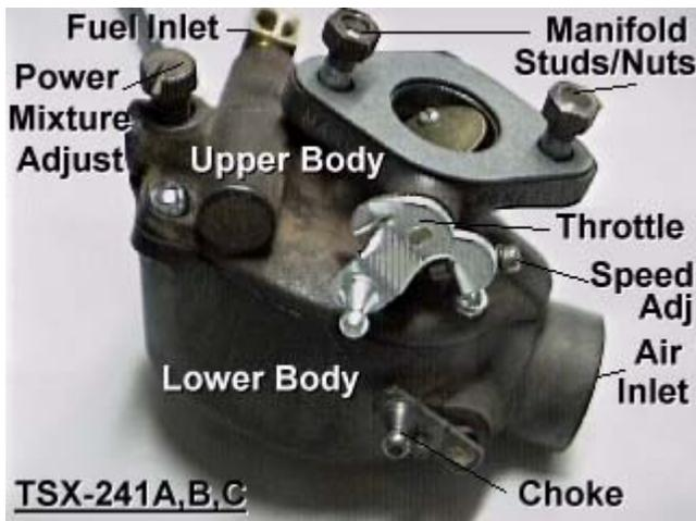
Reinstall the power mixture needle/screw and its new gaskets, and reinstall the idle mixture needle/screw and its new gasket. Screw the two mixture screws closed then back off 1-1/2 turns. Back out the idle speed screw on the throttle shaft until the butterfly fully seats closed.
