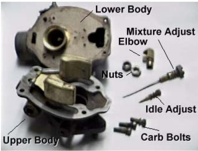
Remove the idle mixture screw/needle, spring and gasket, the power mixture screw/needle, spring and gaskets, and the fuel strainer/elbow.
