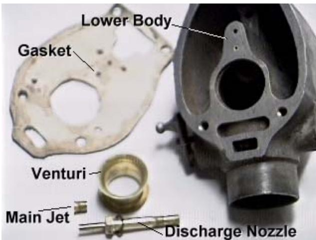
Place the lower body, main jet, and discharge nozzle into the parts basket and lower it into the carburetor cleaner soup.
