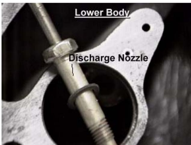
In the cavity under the Main Nozzle is the main jet burried way down in there. It's another one of those straightslot screwdriver jobs again. Pick the widest screwdrive that will fit the slot, secure the lower body casting from moving around and apply constant even pressure on the screwdrive to keep it from slipping and out it will come. If you should gall it up, buy a replacement. Again, annoying, but not too expensive.
