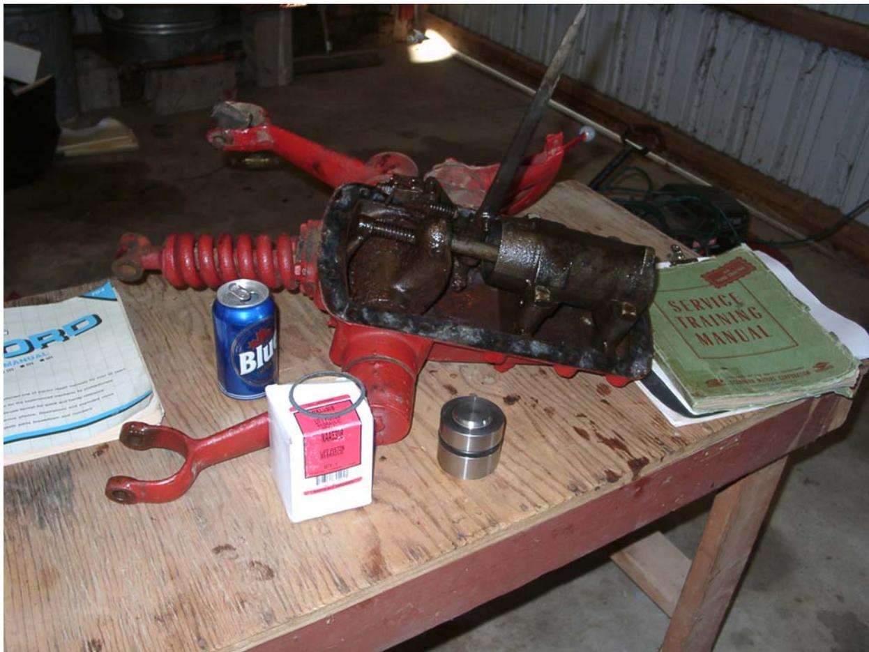
**FIG 5 –Top Cover Removed & On Workbench. Note Control Arm In Vertical Position On Unit.**
