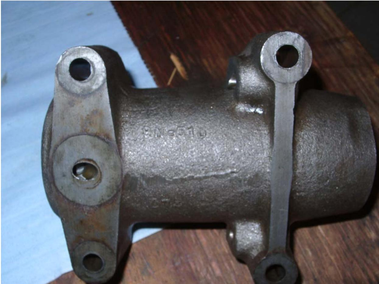
**FIG 8 -The 9N-510-D cylinder from my 8N. Note the part number in raised cast letters & numerals as well as the casting date code below.**
