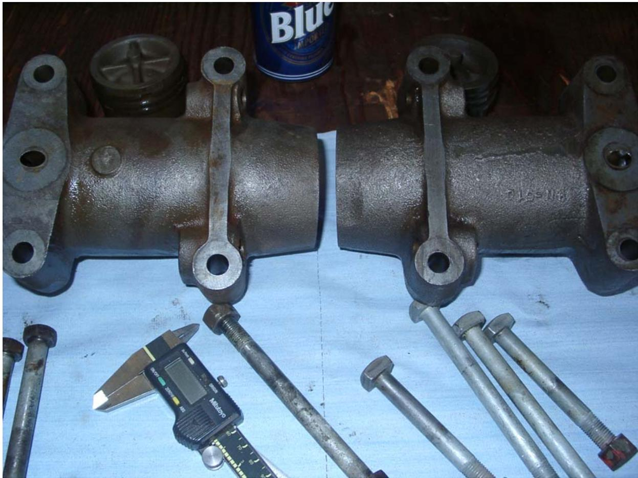
**FIG 10 -Underside of both units –machined dimensions are identical.**
