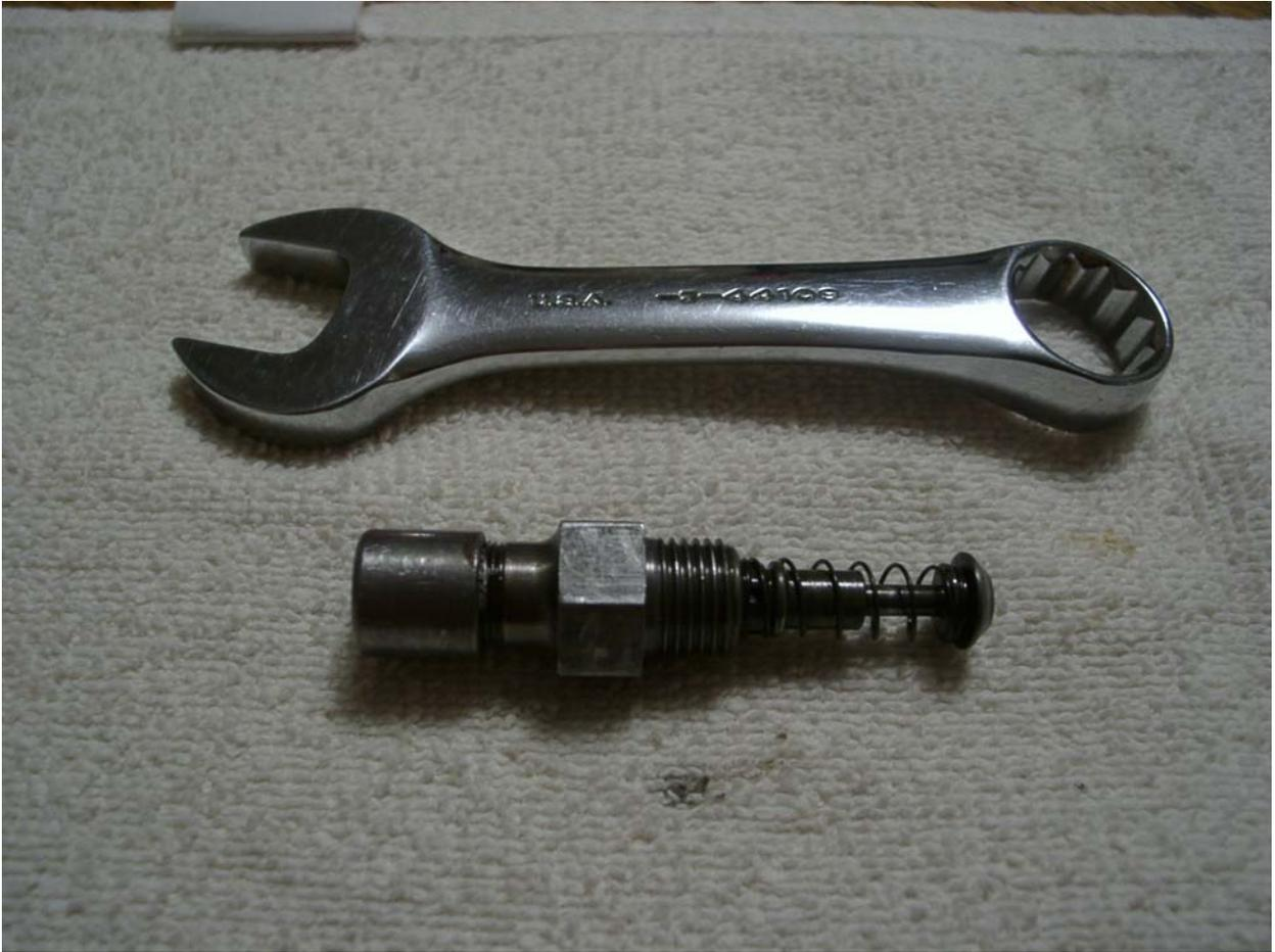
**FIG 00 –Part Number 8N-638, Safety Relief Valve and stub-style wrench.**
