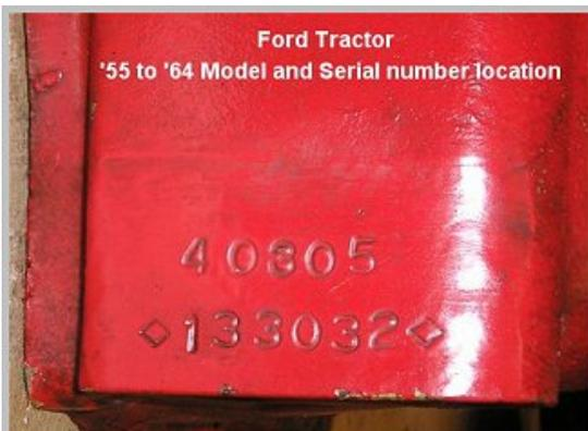
Model and serial number location on early thousand series tractors is the same as the hundred and "01" series tractors.
