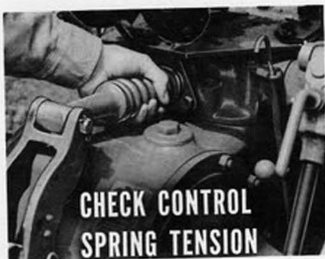
Figure 2 Draft Spring Adjustment
