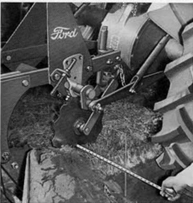
Figure 11 Measuring for Correct Width of Cut
