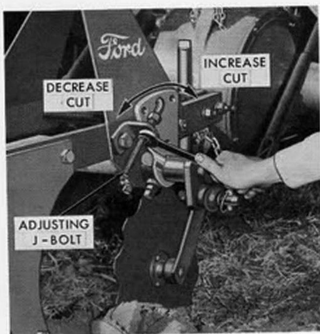
Figure 12 Changing Width of Cut
