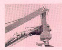
Pat. Pending release clutch shown in disengaged position for raising auger without turning. . . . . . . . . .
