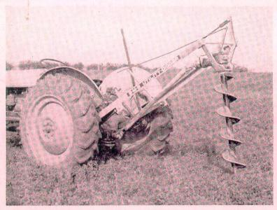
Gear box shown and used is standard Ford or Ferguson belt pulley. Digger is sold as complete unit or less belt pulley.
