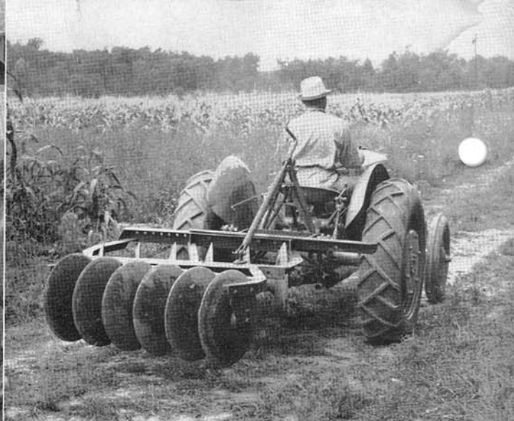
The implement in transport position. Normal clearance between discs and the ground, with harrow lifted for transport, is 6\frac{3}{4} inches. The lift-type design aids both convenience and economy, as wear and tear on the disc blades is eliminated when transporting the harrow on lanes or roads. Transport trucks are unnecessary.
