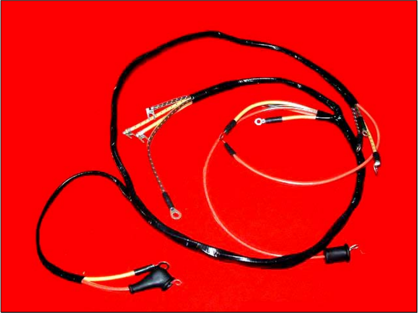
Figure 5 - This is a Dennis Carpenter reproduction of the 8N14401-C main wiring harness. This is a rubber tape wrapped harness used on 8ns with the angle drive distributor after serial number 263843.
