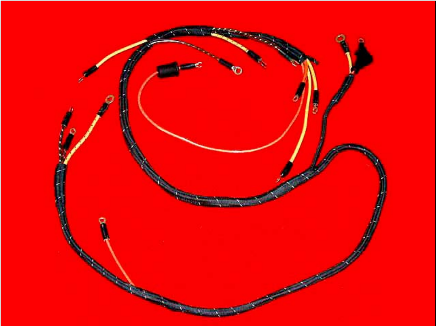
Figure 4 - This is a Dennis Carpenter reproduction of the original cloth wrapped 8N 14401-B main wiring harness which is used on 8Ns with a front mounted distributor up to serial number 263844.
