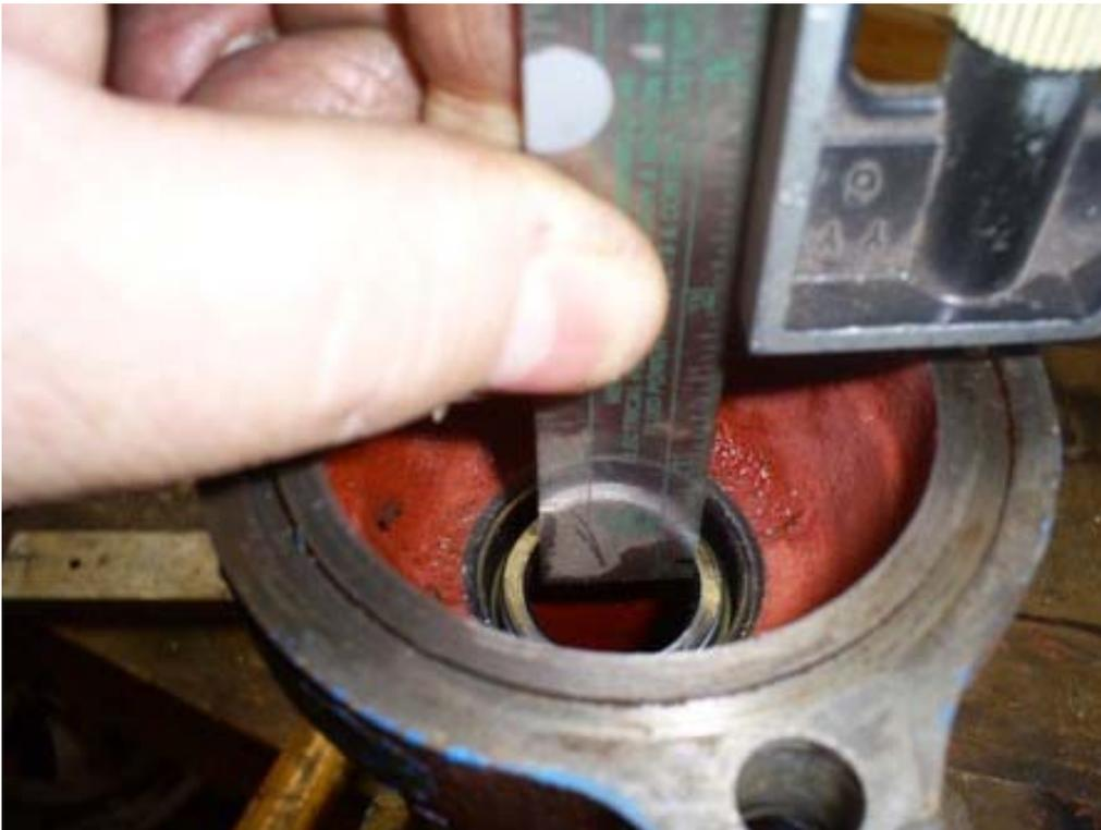
In the following picture, I have driven the new Speedi Sleeve down to just above my marks. From this point on I use a square and a machinist ruler to locate the sleeve. I have also installed the 3 bolts temporarily to hold the bottom block down tight. The photo shows me checking to see if the lip of the new seal lands in the middle of the Speedi-Sleeve.
