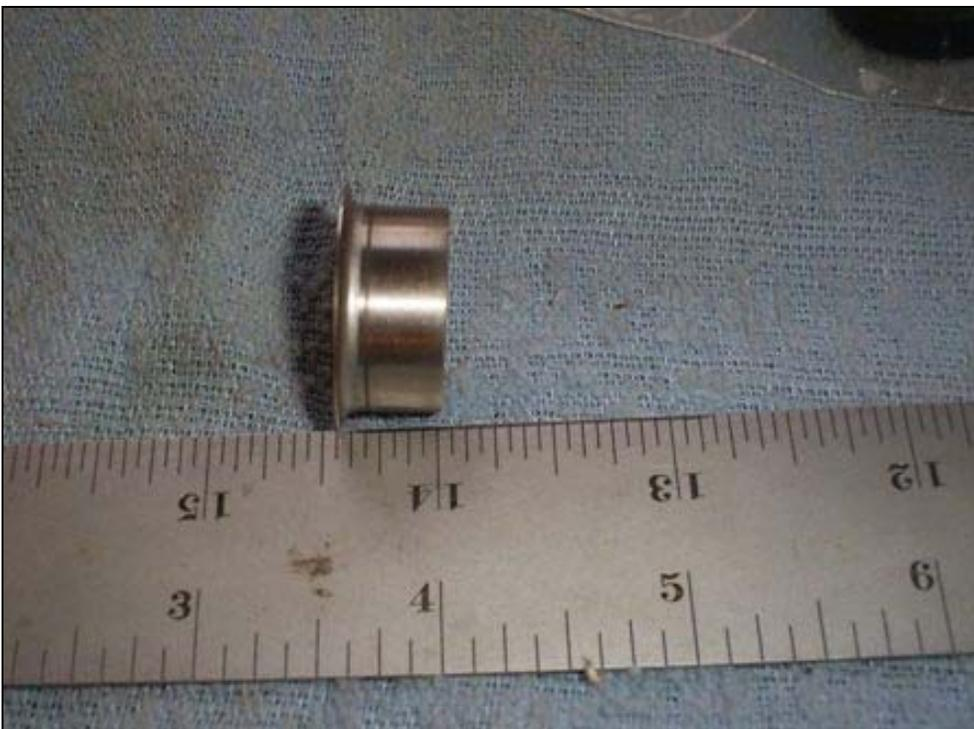
Install the new seal into the upper casting. I used a socket of the same O.D, a short piece of heavy bar stock, and a hammer. Drive carefully and its ok to lube the seal to aid installation. Make sure the seal is completely bottomed out in the casting.
