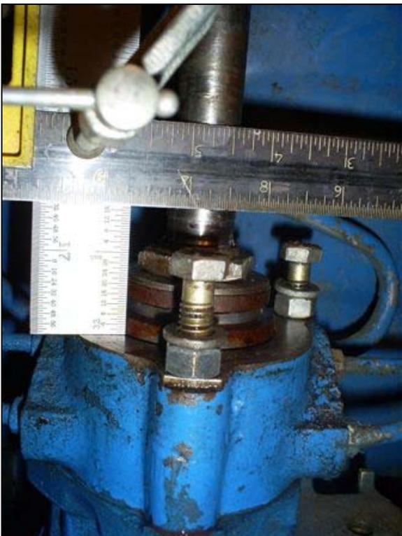
From here I lightly lubricated the new seal and reinstalled the upper casting with the new seal. It dropped onto the shaft and stopped at what I believe is the Speedi-Sleeve where it required just a little force to go on down.
