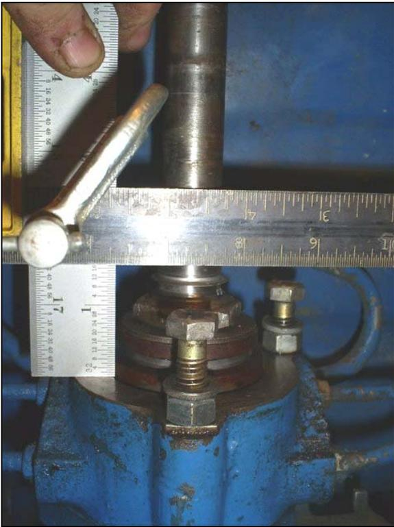
After driving the Speedi Sleeve to the proper location, I removed the flared lip and did a final check, if I've done the math right, the lip on the new seal will land exactly in the middle of the new Speedi Sleeve. Instructions for installing the Speedi-Sleeve were in the seal kit I purchased through YT.
