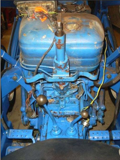
Once the upper casting is removed the lower steering assembly is visible along with the steering shaft that the seal runs against.
