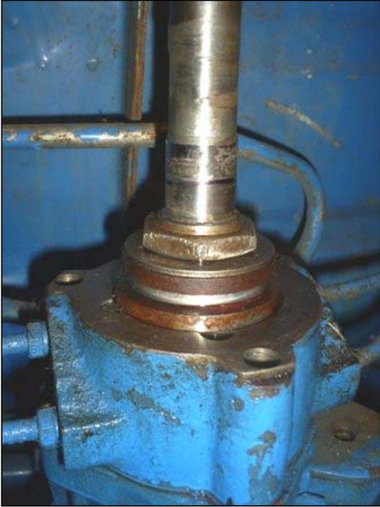
This is a picture of the Speedi Sleeve that came with the kit. It's a very thin machined piece of Stainless steel that provides a new sealing surface without having to re-machine the shaft. It has a flared collar to aid installation that will be removed when completed. The kit comes with a bigger sleeve that fits over this one that you drive against to move the Speedi-Sleeve into position. Notice the groove on the left side near the flair; this is where the flair breaks away when installed.
