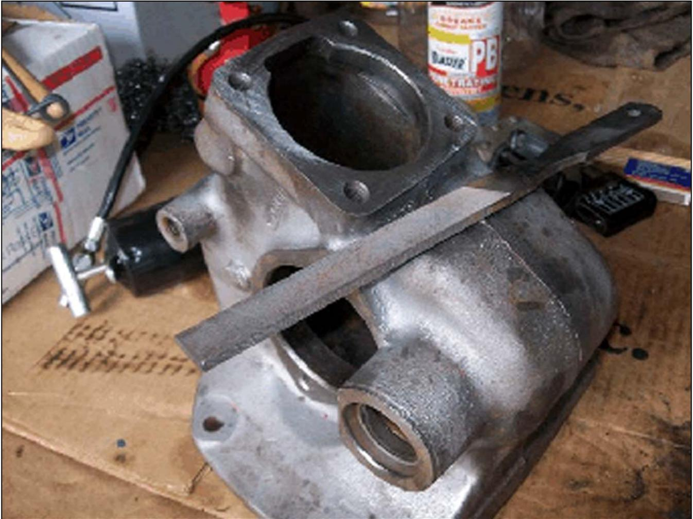
**Step 6** - Inspect the bearing cup seats in both the steering box and the bottom of the tube assembly. No rust or burrs should be present. Remove them with a small wire wheel or small fine grind rock fixed in a drill. Now blow out the box and tube assembly good with compressed air to remove any steel filings.
