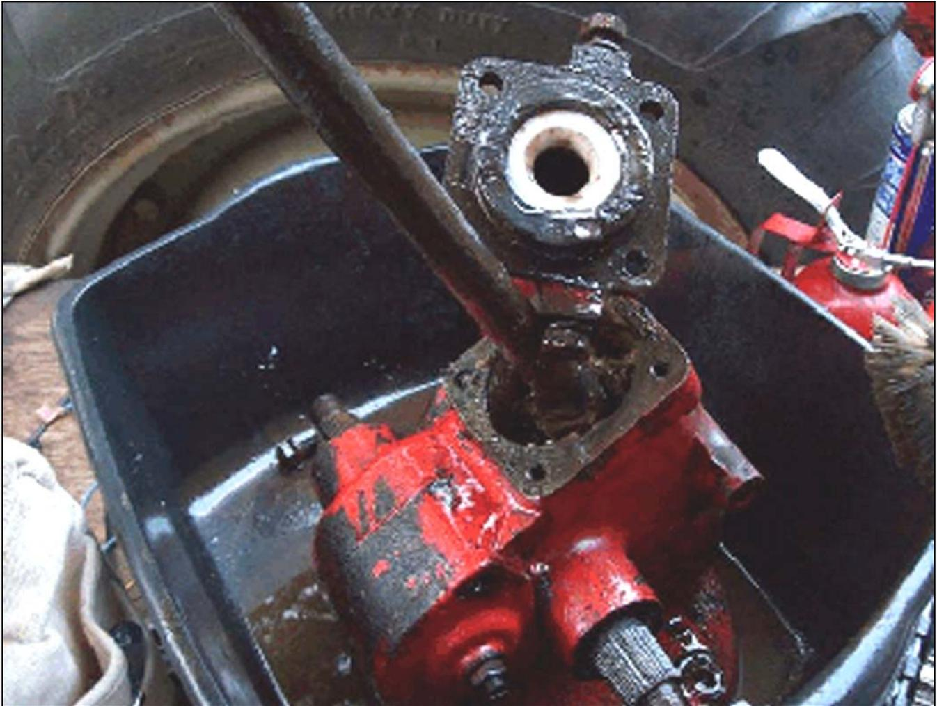
**Step 3** - I then pressure washed all parts, but a good hosing off will do fine. You want the unit as clean as possible. Handle the unit with care and be sure to remove any grit and oil. The last thing you want is to drop the box and crack or break something.
