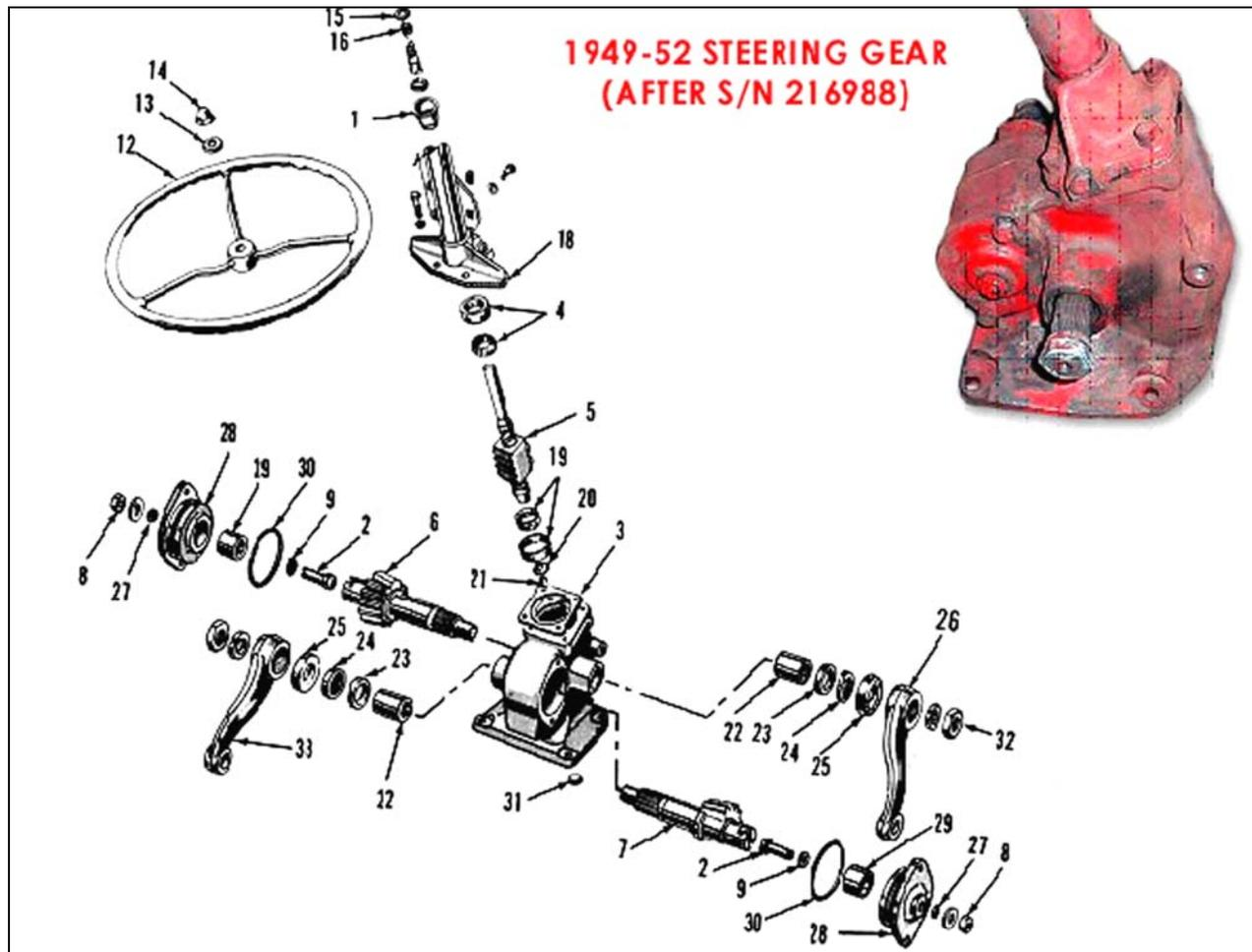
**Keep a print out of "Servicing the Steering Assembly from the FO-4 manual along with this exploded view/diagram of the steering assembly on your workbench for reference.**
