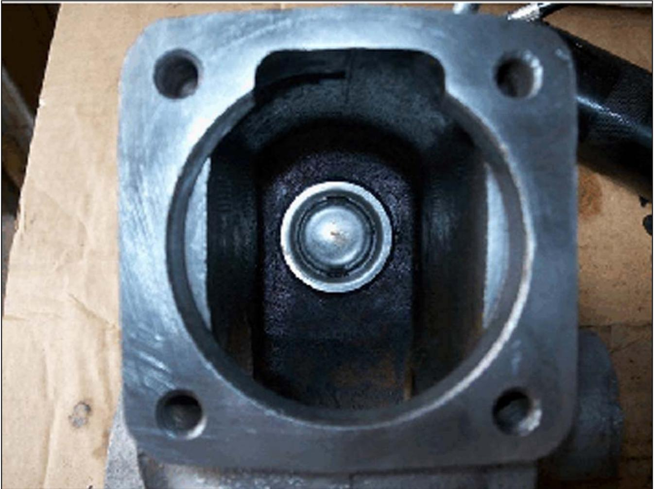
**Step 8** - Drive the bearing cup (8N 3552, thrust bearing cup) into the seat of the tube bottom using the same procedure. Fix the tube assembly in a vise lightly clamped while you work.
