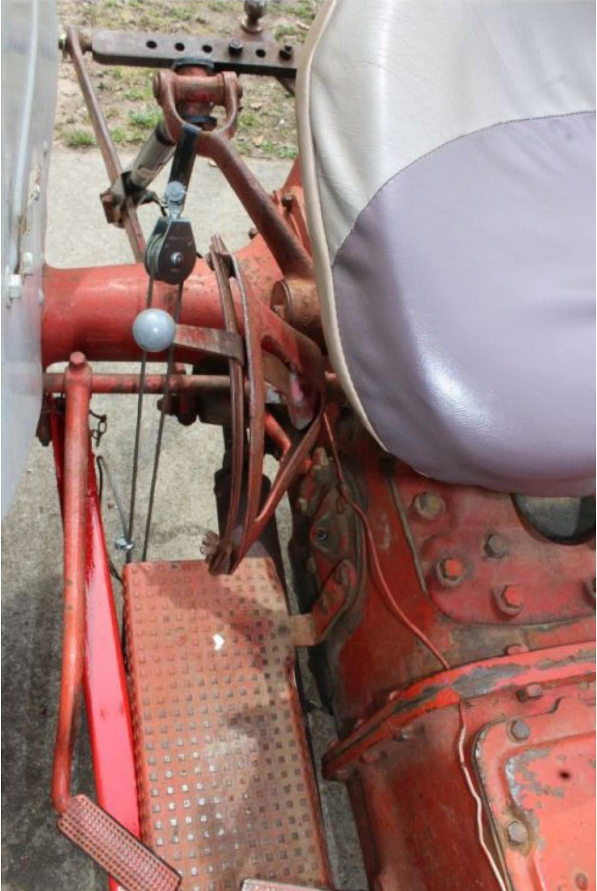
I adjusted the cables so full up raises the blade arms up to the bottom of the bumper. I didn't have much more lift than that anyway.
