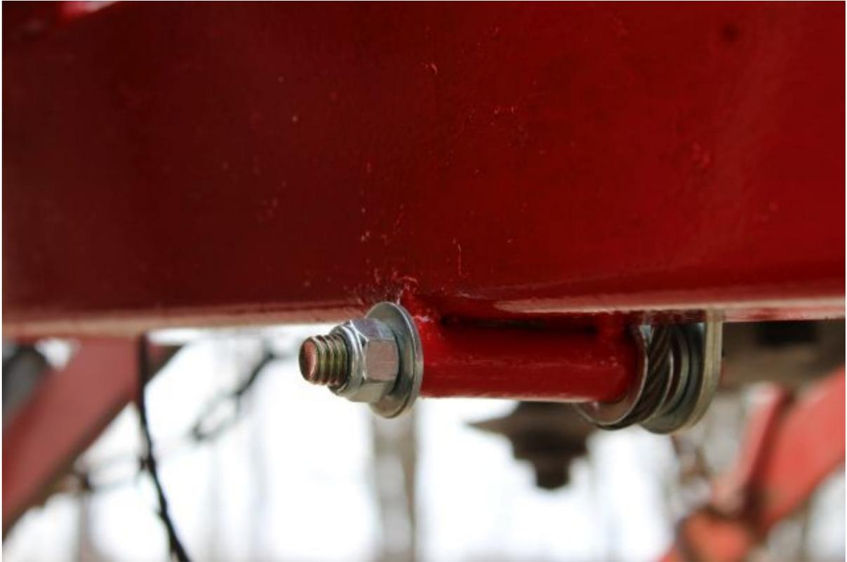
I welded a piece of pipe to mount the cable end thimble and a pulley. It angles to the front a little and extends to the inside about 3/4 inch. I probably could have done without the thimble, and probably should have angled the inside end of it down to hold the pulley at a better angle for the cable but just leaving the lock-nut a little loose lets the pulley lean and it works fine.
