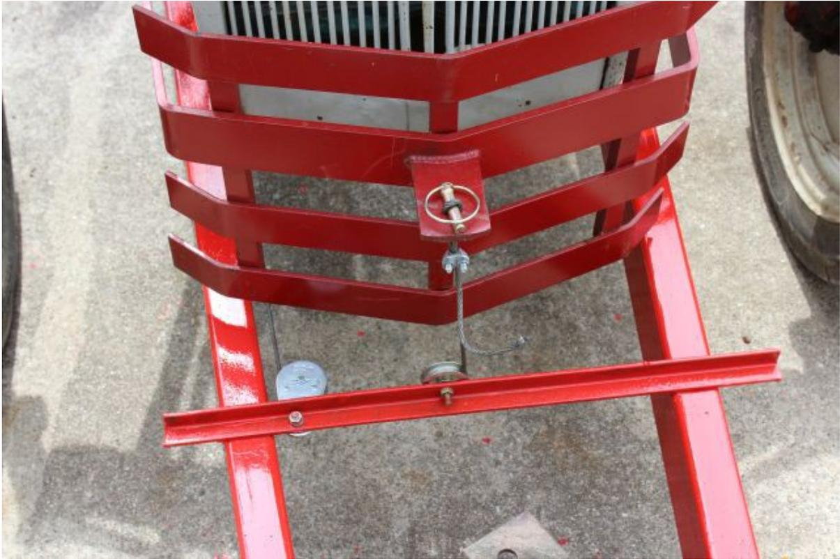
I took one of the swivel pulleys apart for the wheel. I drilled and tapped the holes for the bolts and added a nut to lock the bolt in place so the wheel would turn.
