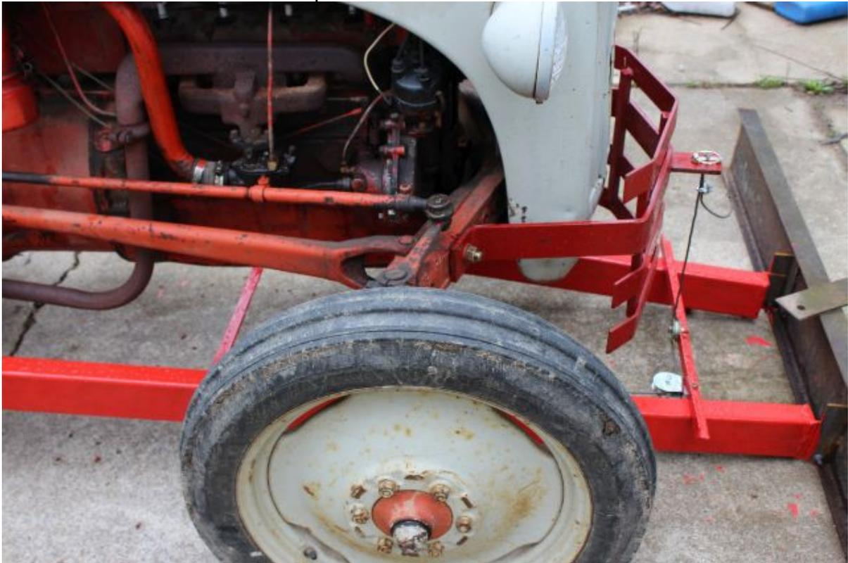
Here you can see the cross brace under the motor. This was a mistake, I should have angled it towards the front to triangulate it. Plus I need a long heavy bar in the back of the arms to bend them in enough to go onto the mounting pins.
