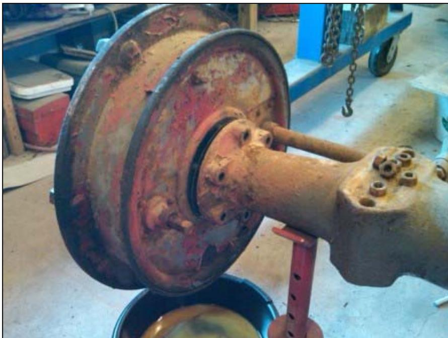
The brake backer plate may come out with or without the brake drum and it doesn't matter. I chose to separate the backer plate from the drum as it comes off the tractor as it's a little lighter that way. Have a long bolt or something handy to shove through the axle and backer plate if you wish to leave it on the tractor.
