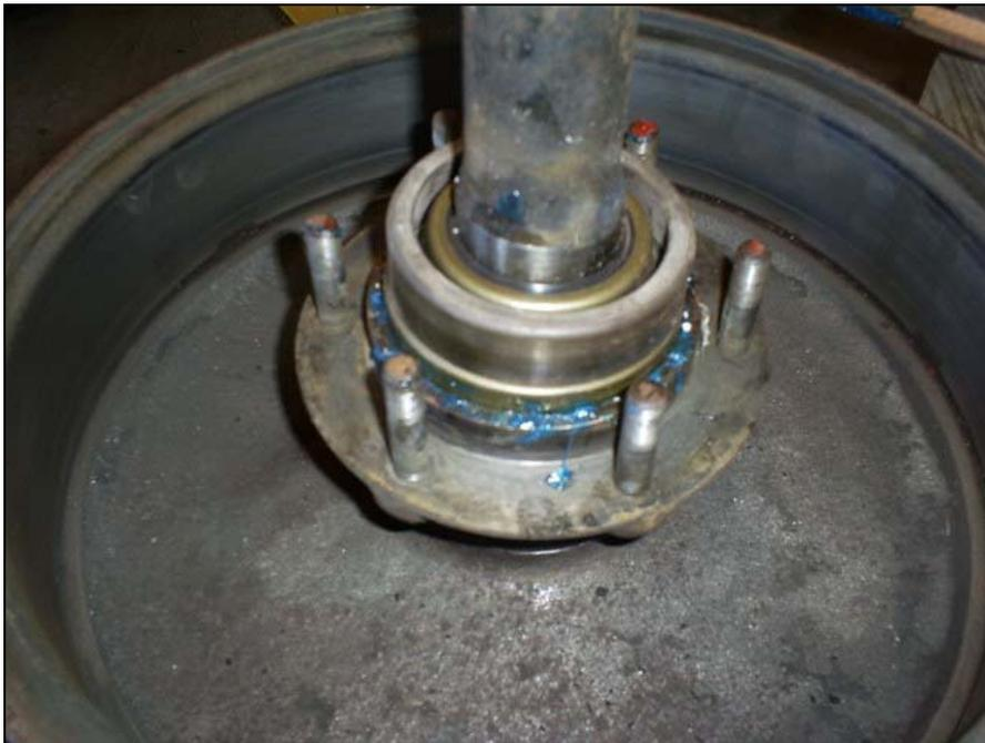
Drive the Sure Seal down until it's flush with the bearing retainer casting and clean up any remaining grease. Pull the bearing retainer up and rotate and see if the seal is running true or moving about the shaft indicating that the seal is not square with the shaft.
