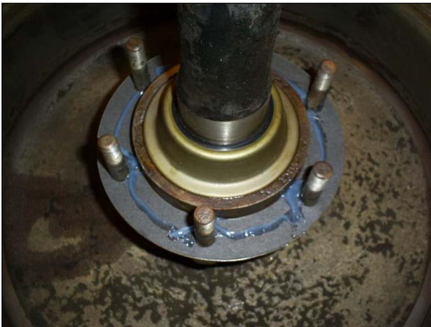
Slip the brake backer plate with the brakes installed into the brake hub.
