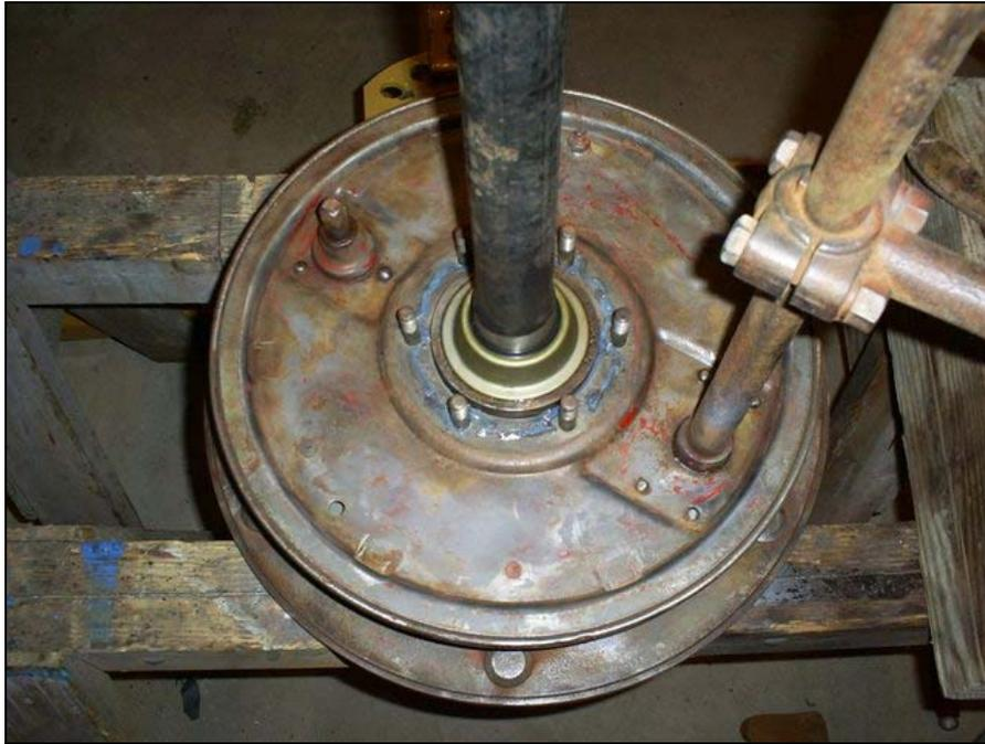
Slide the axle and brake backer plate into position on the tractor, make sure the brake cross shaft is seated in trumpet casting and tighten the 6 nuts. You may have to rotate the hob to get the axle to slide into the differential. You can see the silicone oozing out, this should be a very good seal. Test to see that the hub still rotates and that the brake works. You will adjust the brakes later.
