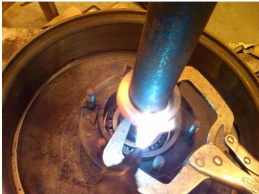
Here is the new collar installed. Polish the shoulder of the axle with 400 grit emery cloth just ahead of the collar as this is where the sure seal forms its seal. Damage to this area has to be repaired if using sure seals.
