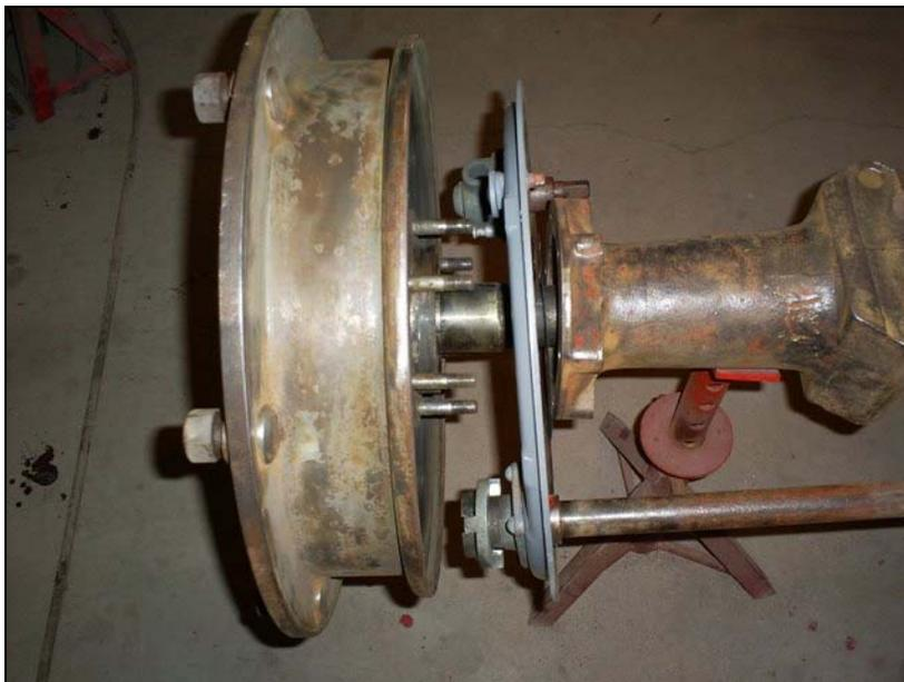
To install the brakes, mount the backer plate on a firm surface, I use the tractor axle. I have a couple bolts in place to keep it from moving. Start by hooking the blue spring on the shoes then place end on the non-adjuster end. Once the ends are in place it's easy to lift the other end of the shoes over and into the adjuster. Once in place add the retainer clips. Make sure that the pads seat down into the brake adjuster plungers correctly.
