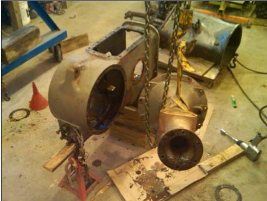
With the left trumpet off, reach in and remove the differential. This is another very heavy part. Take care not to drop it. Place several layers of heavy cardboard on the floor in case you do. Once out inspect the ring gear, bearings, the bolts, and the rivets that fasten the ring gear to the carrier. Broken rivets are not uncommon and there are bolt kits available to replace them.
