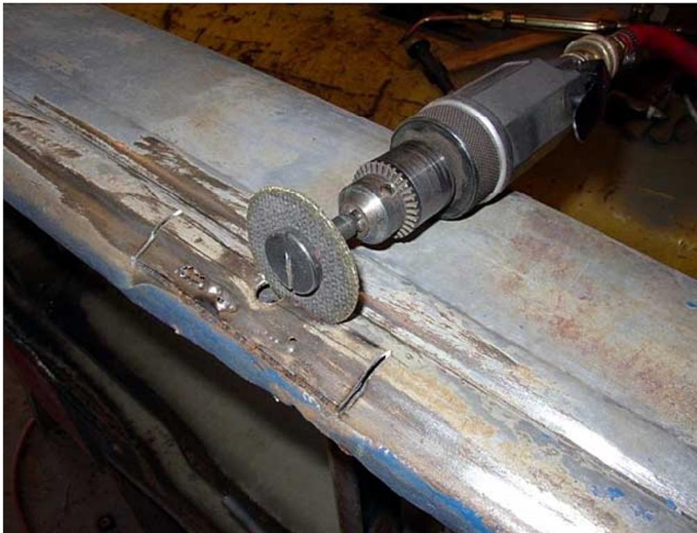
Make a filler piece. I use an old Ferguson hood which has similar rib features. I spend time with the bench vise and a hammer shaping the piece to match the contour. A tight fit is best. You could also use an old fender/. The steel is about the same thickness.
