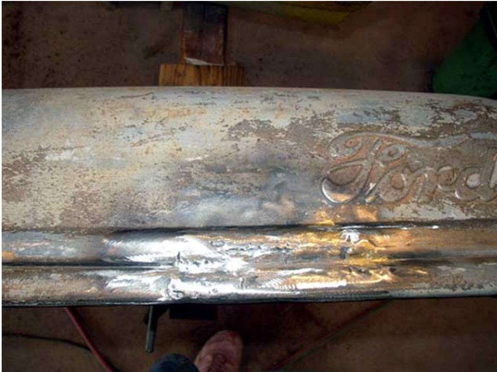
Check the repair and make sure it is not higher than the surrounding metal. I hammer the high spots down. High spots will be visible when painted.
