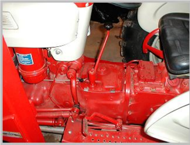
The 5 speed transmission shifter Used 1955 - 1964
