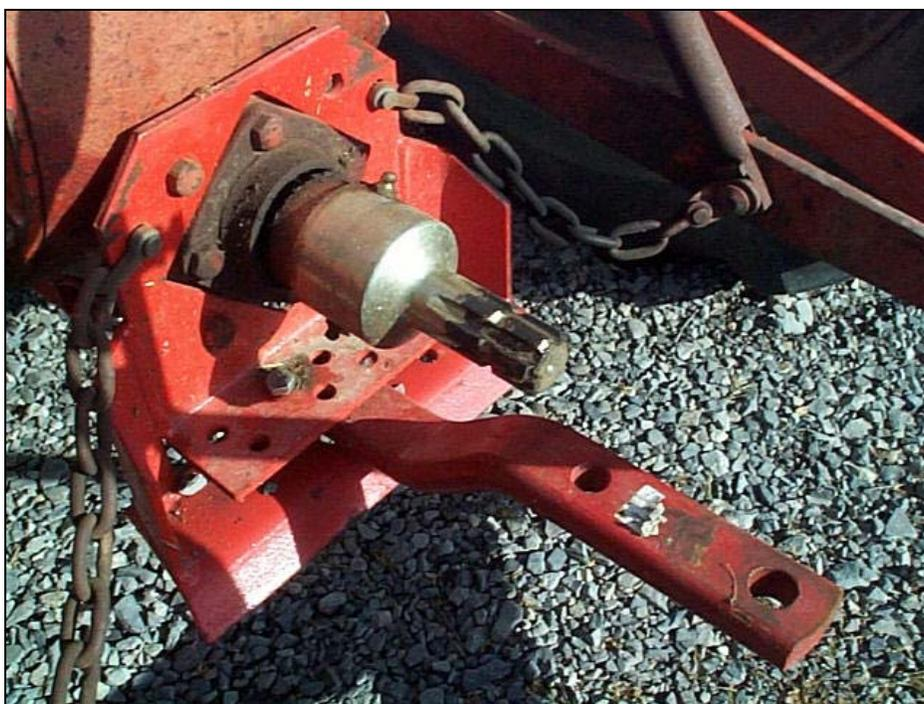
The most practical thing about the generic type of swinging drawbar setup is that you can leave it on, (most of the time anyway), and still hook up other 3-point implements. I only remove mine when using a PTO-driven implement (mower, post-hole digger, etc.).
