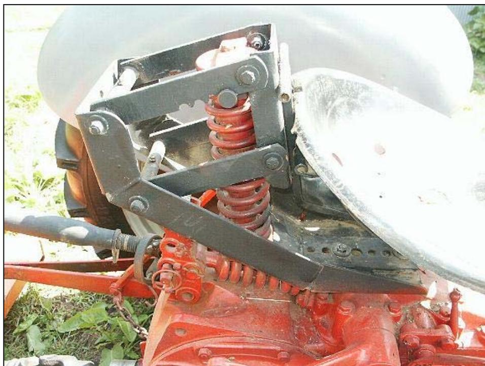
I bent the metal seat roll down where the seat fits as far back as possible, hard against the mounting plate.
