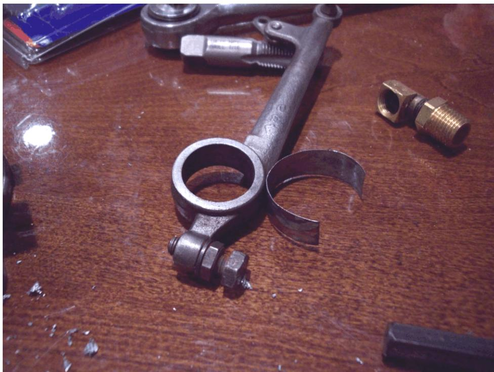
Be sure to flatten the face of the body as the related governor article in the NTC's "How-To" section describes. Do **not** over tighten the bolts, and **make sure the short bolt goes back in the top hole.**
