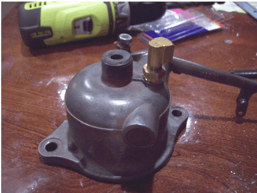
While I had the arms off my governor, it was a good time to repair the wobble that is so common with these governors. I cut a strip from an aluminum soda can, greased it and wrapped it inside the lever (9N18190 (9N, 2N) or 8N18190 (8N)) as a shim and re-assembled the governor.
