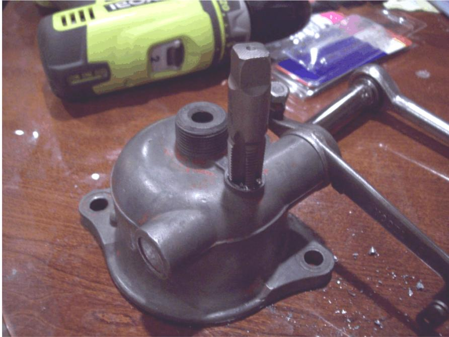
Take the 1/4" MIP x 1/8" FIP bushing and anchor it in your vise. Saw off approximately 3/16" of the male end. This fitting will bottom out against the lever rod and fork and prohibit it from rotating properly. After you have sawed the end off, dress it on your grinding wheel and brush it clean. Wrap the threads in Teflon tape and tighten it into the governor housing. Next, wrap the original elbow 87381S in Teflon tape and tighten it into the bushing. Fitting cost about \$2.00
