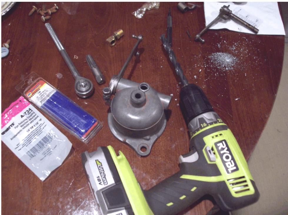
Tap the freshly drilled hole with a 1/4" x 18 NPT tap. Extreme care must be taken here to keep the tap straight and aligned with the hole, as well as keeping downward pressure. Use cutting oil. (Pot metal will shear much quicker than steel.) Tap cost \$5.29
