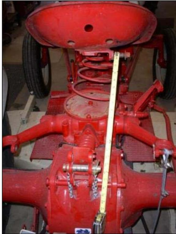
The seat was check extended and compressed looking for the right place to relocate the upper mount.
