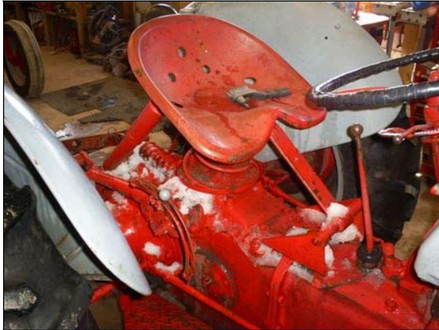
This is the rear view. The rear shock has a special bracket that bolts to the rear differential.
