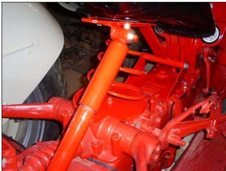
And here is the rear view. The new shock came with rubber bushings that were a tight fit on the long pin. I also made spacers to take up the available space on the mounting pin so that the shock will stay put. The spacers were made from a 3 pt bushing used to reduce holes from Cat 2 to Cat 1 specifications and fit acceptably. I used SAE washers next to the rubber bushings in the lower shock mount.
