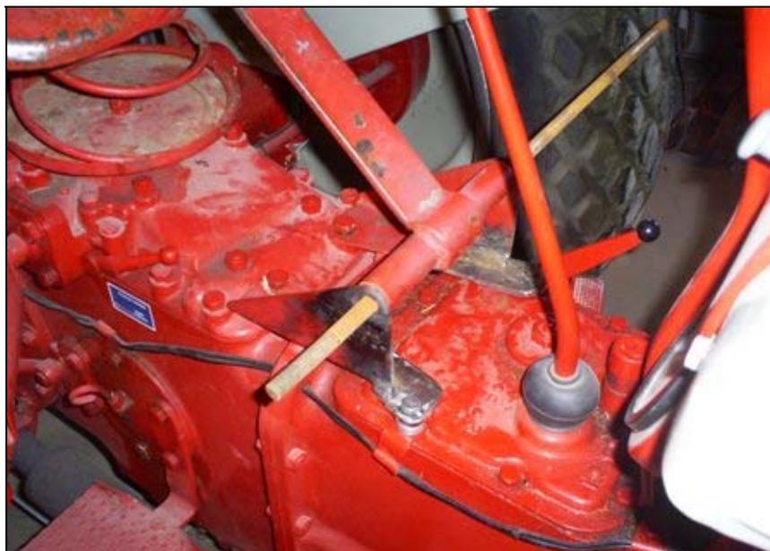
The only available location on the rear casting for the shock mount is the long pin on the pivot for the 3pt spring. I tested this as a location and it appeared ok but upon measuring the stroke of the shock the seat sat too high and would not compress down to level.
