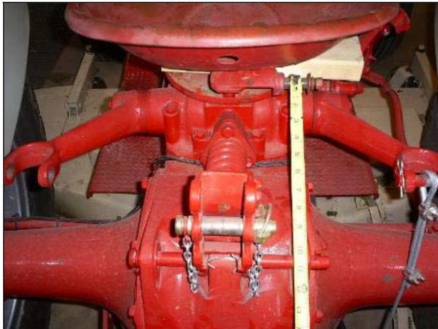
A location was determined that allowed the seat to fully compress just as it bottomed out and worked for the fully extended position. The upper mount was cut off and relocated to its new location. I had to move it from the top of its mount to the underside to clear the seat. I also moved it to the left to allow for the shock to center in the space available on the lower mount.
