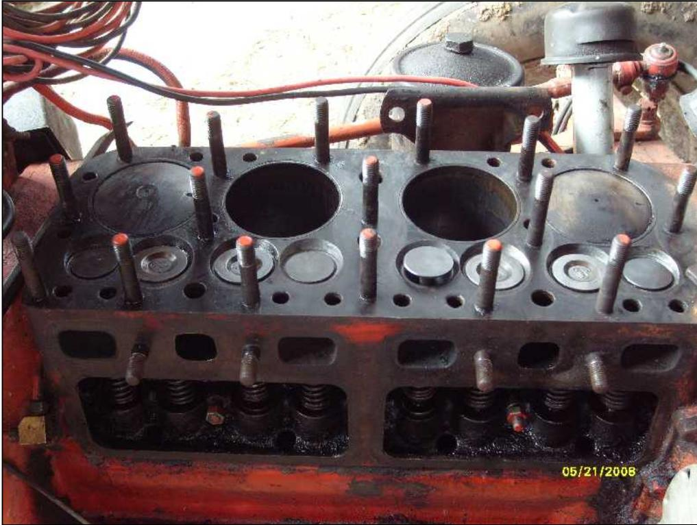
**Step Two:** Get the old parts out. One valve was broke clean in half and I wanted to convert it over to adjustable lifters so I just used a big pry bar get all the old valve guides out.
