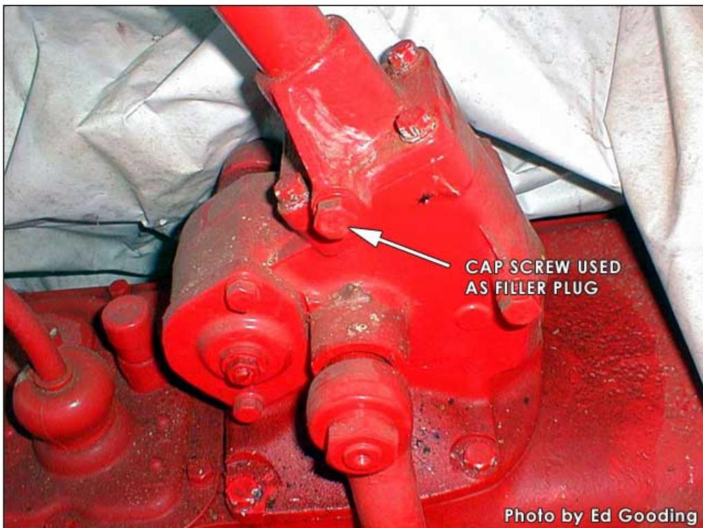
The housing should always be filled to the level of the cap screw hole to insure that the top bearing (8N-3571), receives lubrication. Fill when the level falls below the cap screw.
